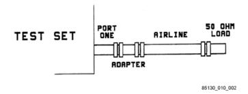
Return loss is measured by connecting a 50 ohm fixed load termination through a 5.0 cm airline to the adapter, then attaching the adapter to port one of the test set (see Figure 2).
